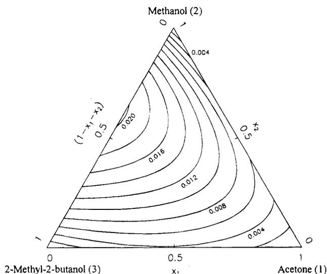
**Figure 5.** Changes of refractive index on mixing curves for acetone (1) + methanol (2) + 2-methyl-2-butanol (3) mixtures at 298.15 K.
