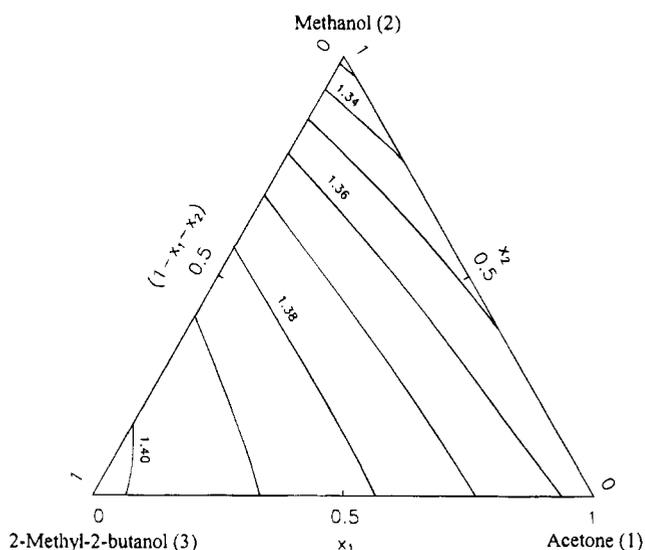
**Figure 3.** Refractive index curves for acetone (1) + methanol (2) + 2-methyl-2-butanol (3) mixtures at 298.15 K.
