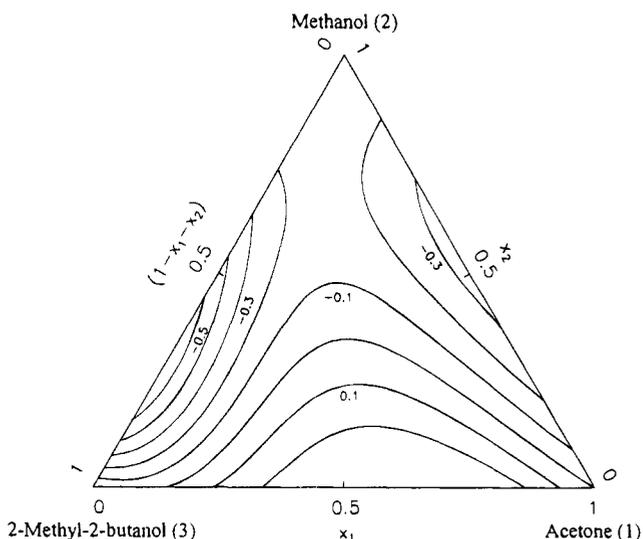
**Figure 4.** Excess molar volume curves for acetone (1) + methanol (2) + 2-methyl-2-butanol (3) mixtures at 298.15 K.
