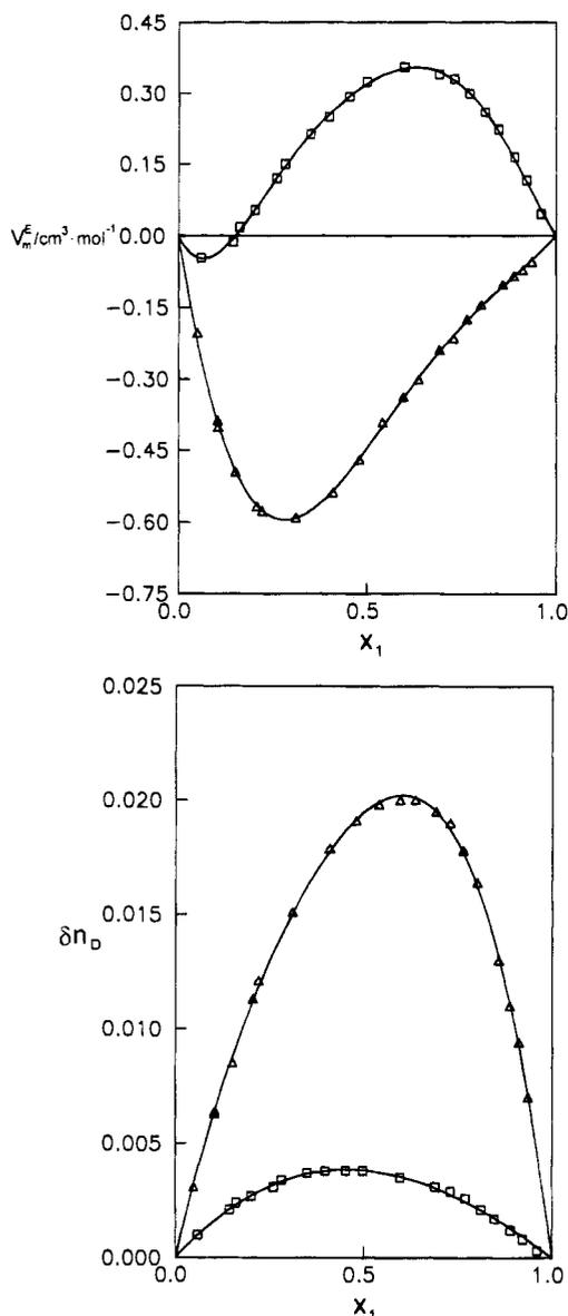
**Figure 1.** Variation of the (a, top) excess molar volumes and (b, bottom) changes of refractive indices on mixing with mole fraction at 298.15 for (□) acetone (1) + 2-methyl-2-butanol (2) and (Δ) methanol (1) + 2-methyl-2-butanol (2).
