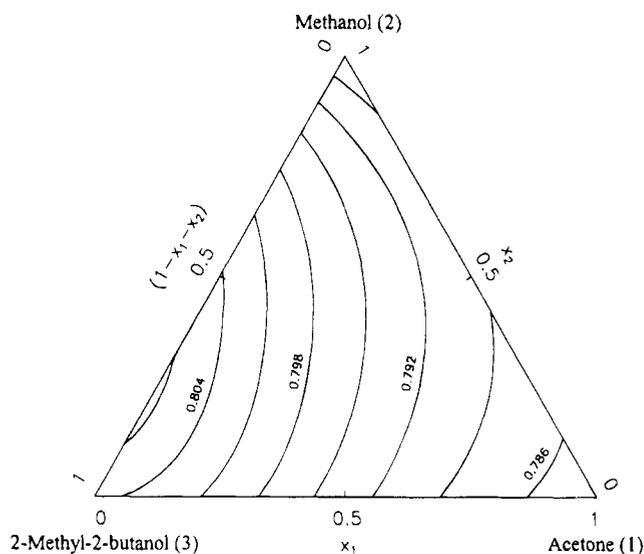
**Figure 2.** Density curves for acetone (1) + methanol (2) + 2-methyl-2-butanol (3) mixtures at 298.15 K.
